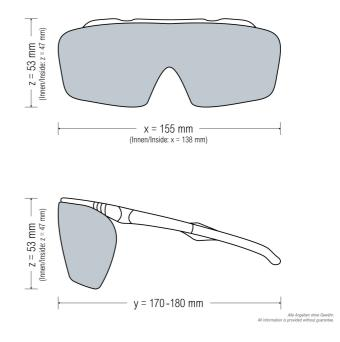
Laser safety goggles with special yellow plastic filter suitable for Excimer (193 nm), UV (248 nm), Nd:YAG 4x (266 nm), Nd:YAG 3x (355 nm), Blue light laser (450 - 480 nm) and Diode (450 nm) laser
