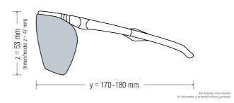
Laser safety goggles with gray plastic filter, suitable for Ho:YAG (2100 nm), Thulium (1480 + 1940 nm), Er:glass (1540 nm) and Telecom (1320 nm) lasers
