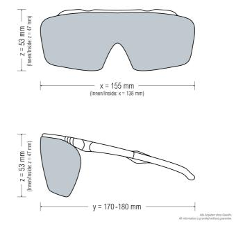
Laser safety goggles with blue plastic filter, suitable for diode (630-660 nm) and He:Ne (633 nm) laser
