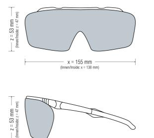
Laser safety goggles with magenta plastic filter, suitable for Dye (577 nm) laser
