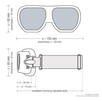
Laser safety goggles with light grey mineral glass suitable for Yb:YAG/Disc (1030 nm), Nd:YAG (1064 nm) and Fiber (976 - 1080 nm) lasers
