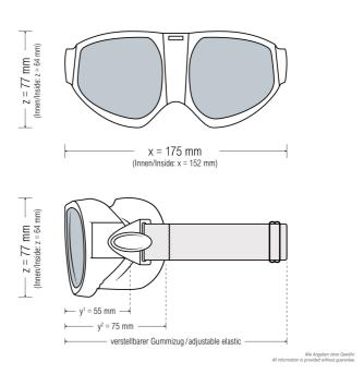
Laser safety goggles with orange mineral glass suitable for Excimer (193 nm), UV (248 nm), Diode (450, 480 nm), harmonic Nd:YAG (266 nm + 355 nm + 532 nm), and Argon (515 nm) KTP (532 nm) lasers
