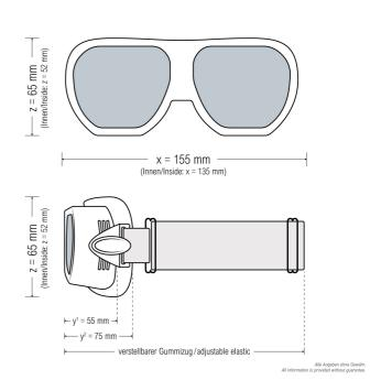
Laser safety goggles with light gray mineral glass suitable for Diode (980 nm), Yb:YAG/Disk (1030 nm), Nd:YAG (1064 nm), Fiber (976 - 1080 nm), Telecom (1550 nm), Ho:YAG (2100 nm), Er:YAG (2940 nm) and CO2 (10600 nm) lasers
