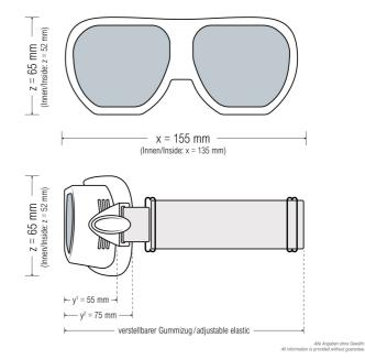
Laser safety goggles with light gray mineral glass suitable for Diode (980 nm), Yb:YAG/Disk (1030 nm), Nd:YAG (1064 nm), Fiber (976 - 1080 nm), Telecom (1550 nm), Ho:YAG (2100 nm), Er:YAG (2940 nm) and CO2 (10600 nm) lasers
