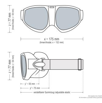
Laser safety goggles made of special green plastic suitable for Diode (630 - 660 nm), He:Ne (633 nm) and adjusment (EN 208) lasers
