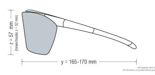
Laser alignment glasses with special gray plastic suitable for alignment (400-700 nm) laser
