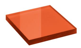
Laser protection window made of special orange plastic suitable Excimer (193 nm), UV (248 nm), Nd:YAG 3x (355 nm), Nd:YAG 2x (532 nm), Diode (450 nm), Diode (480 nm), Argon (515 nm) and KTP (532 nm) lasers
