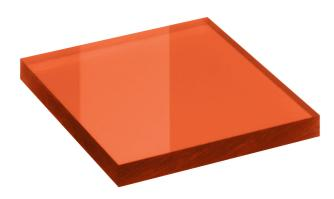
Laser protection window made of special orange plastic suitable Excimer (193 nm), UV (248 nm), Nd:YAG 3x (355 nm), Nd:YAG 2x (532 nm), Diode (450 nm), Diode (480 nm), Argon (515 nm) and KTP (532 nm) lasers
