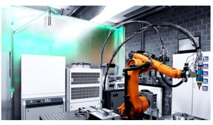
Smart Shield is a retrofittable, fully automated laser protection system facing the laser that uses the existing protective wall as passive protection for the duration of the shutdown process.
